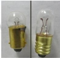
Replacement/reproduction is bayonet style PN 243004V Corbin speedometer bulb 1938-47, 1952-53. Original is threaded style PN 10683V
